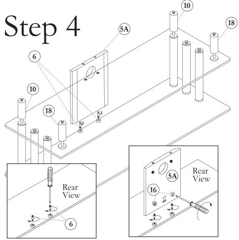
A - Insert & Tighten Cam Bolts (6) into round metal nuts mounted on the top glass shelf
